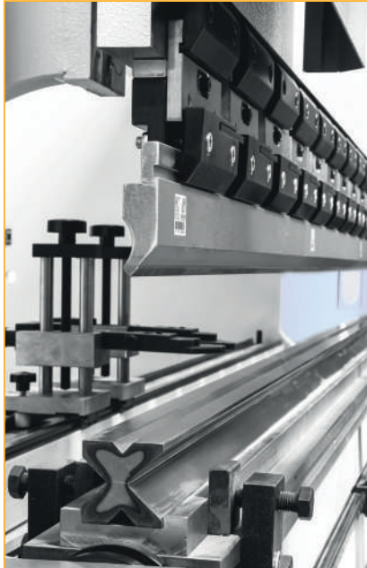
European type separated top and bottom tools system from Eurostamp or Roller (standard)
